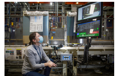
Lana Chausenko, an engineer on our new Industry 4.0 Development Program, works with the camera used to detect leaks on the dishwasher test loop. Incorporating vision or cameras is a key element of the robotics and automation rotation that is driving expanded flexibility and new capabilities in our Louisville, Ky. plant.
